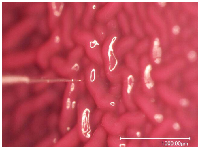
Figure 1: MicroProfiling setup (left) and microsensor inserted into a P. aeruginosa colony (right).
