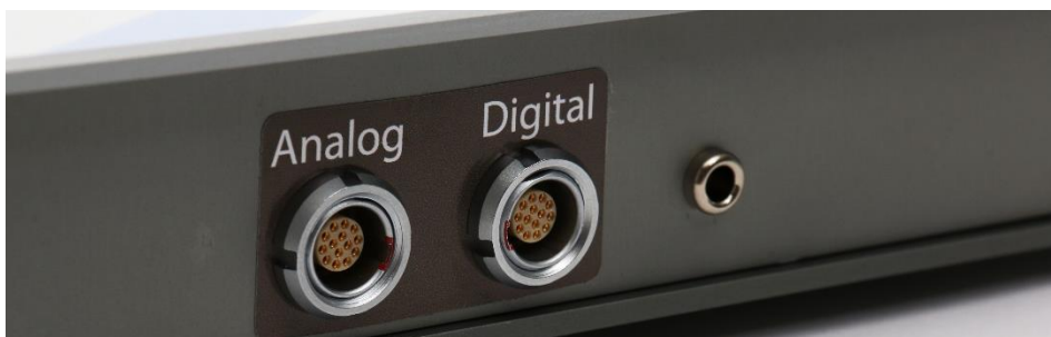
Figure 5: Connectors for Analog and Digital in and output and for the grounding cable (right).
