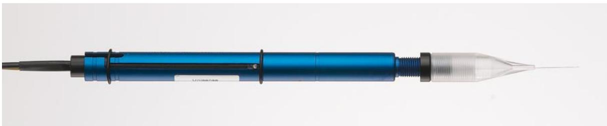
Figure 3: Redox microsensor in the Microrespiration guide.
