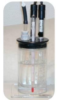
CAL300 with microensors and bubbling with air.
